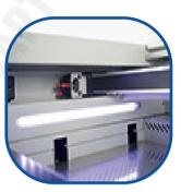
Clean pack design, protect linear guide rail from dust, reduce maintenance frequency
