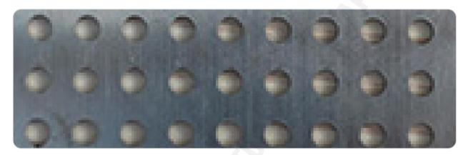
**Sprint laser piercing:** This helps to keep the optics clean and improves the cutting process by pushing vaporized and liquified material out through the kerf, especially for the thick sheet metal.
