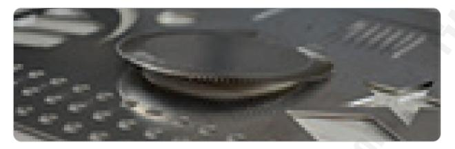
Flying cut: especially for thin metal sheet, fast cut of matrix patterns.
